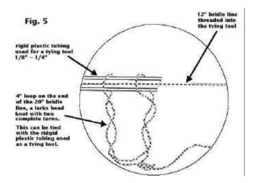
end of the rigid tubing. Slide the twisted loop onto the bridle leg and slide the tubing back off. Pass the loose end of the bridle line through the skin around the last upper bridle point and pull out the slack till the bridle line will no longer reach the wingtips. Secure the knot and use super glue on all none adjustable knots. (See Fig. # 6)
